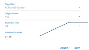
The "PosCtrl" is satisfied if an amplification curve is present. This can be set by defining the requirement for a Ct value lower than the number of cycles planned in the analysis (*e.g.* 40 cycles).
